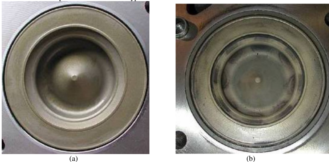
Fig5. The engine piston of Cummins ISB-305 coated with HTP TBC (a) before and (b) after the engine test [38]
